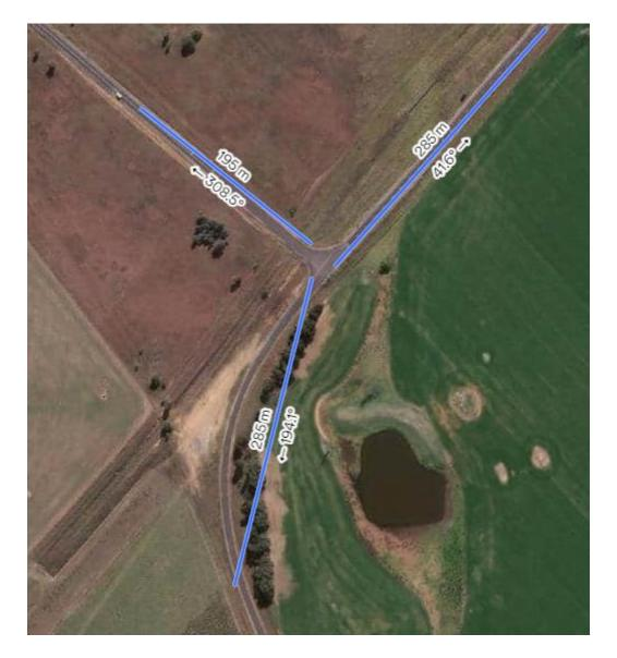
Sight distance from the southern approach is restricted. However, mitigation measures have been installed on the western Cunningar Road approach in the form of raised rumble bars and signage as shown in Figure 10.
