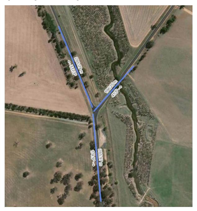
The sight distance from the southern and eastern approaches is adequate. However, the sight distance from the northern approach is restricted by the horizontal and vertical alignment.
